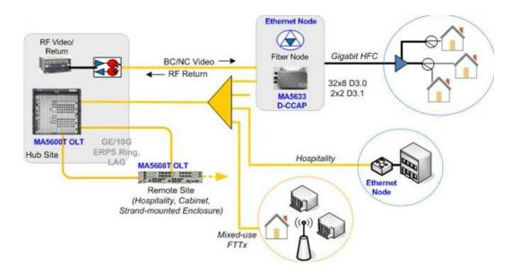
With GPON, 10G GPON, GE or 10GE uplink, Huawei's MA5633 D-CCAP delivers cost-effective, Gigabit bandwidth over existing coax infrastructure in various HFC migration applications. Flexible networking and deployment scenarios including:
